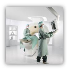
The HIFU table will be upgraded in the next few months. The Philips Sonalleve MR-HIFU device upgrade to Version 2.0 for the Achieve 3.0T includes a new trolley (which replaces a standard diagnostic table top on an MRI machine), a new HIFU transducer, a new RF coils system, new filter panels, and upgraded software.
